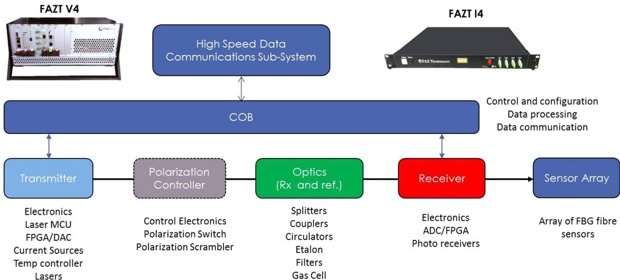
Figure 1. Block diagram of the FAZT tunable laser interrogator
