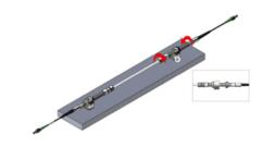
Mount the T230 Sensor into the T230 Brackets by Use a thread securing adhesive (such as Loctite 2701) after moving the washers and nuts to the sides in a way that sensor is fixed and pre-strained in the Mounting Brackets. ensures there is one nut and one washer on each side of each bracket. Leave thread space for pre-straining the
